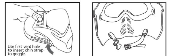
INSTALL CHIN STRAP - Loop around and snap the chin strap (on both sides)
